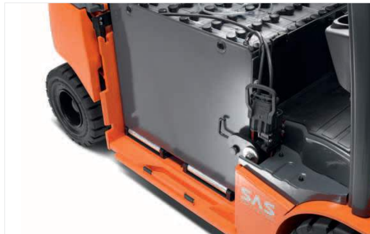
Battery mounted on optional rollerbed for easy extraction. Alternatively, fork pockets allow another forklift to remove the battery
