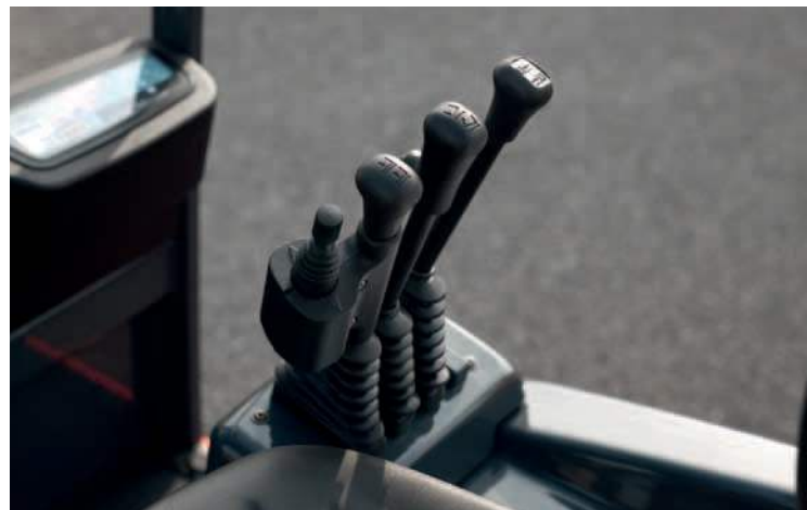
Driver side levers with direction switch come as standard on the trucks.
