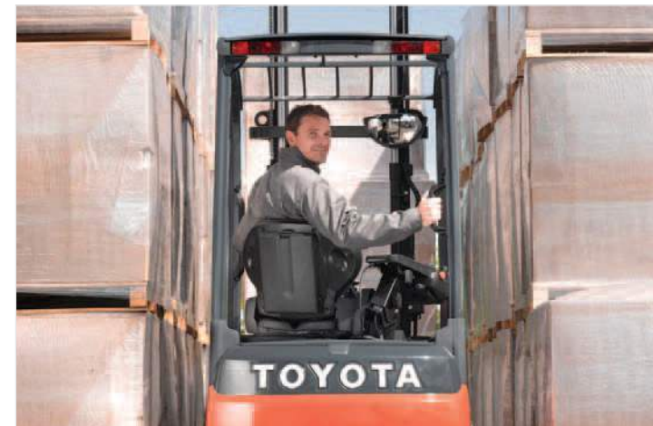
Rear-assist grip enhances reverse travel comfort and productivity by reducing operator back strain. Optional swivel seat aids comfort reversing and getting in and out
