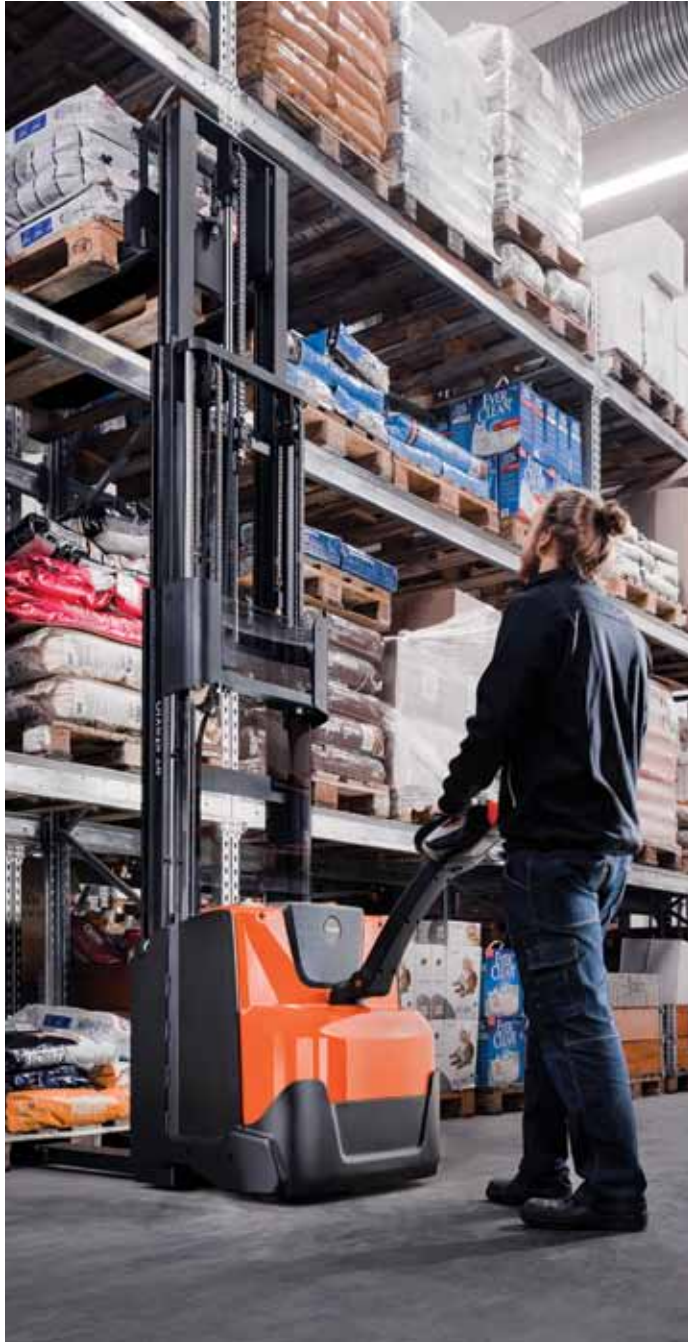
The tiller arm length is optimised for safety, keeping the operator's feet away from the truck
