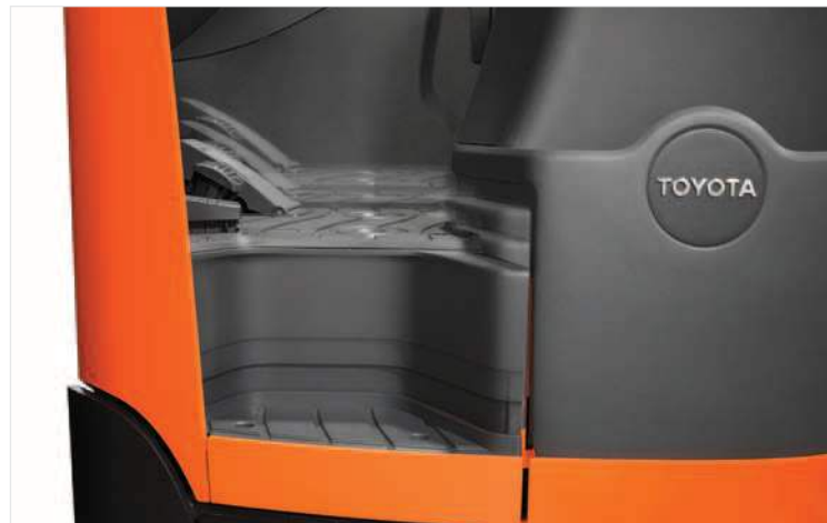
The operator compartment is adjustable to suit different operator sizes. The floor height can be adapted manually or electronically.
