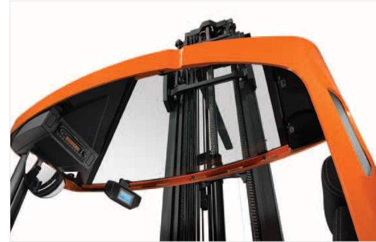
The transparent roof provides a clear upward view to the forks when working at height.
