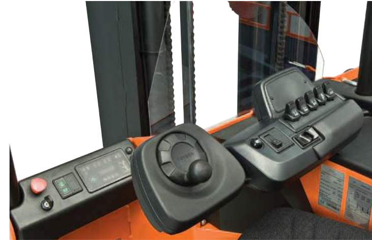
The operator faces the forks to obtain the best view of long and unusual loads
