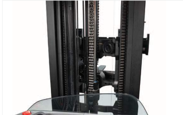
The open fork carriage with integrated side shift offers excellent visibility forward.
