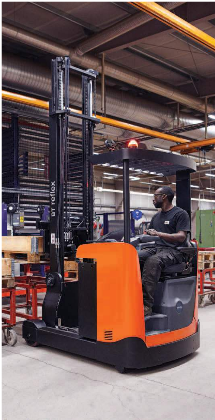
The driver compartment is adjustable to suit different driver sizes. The floor height can be adapted manually or electronically.
