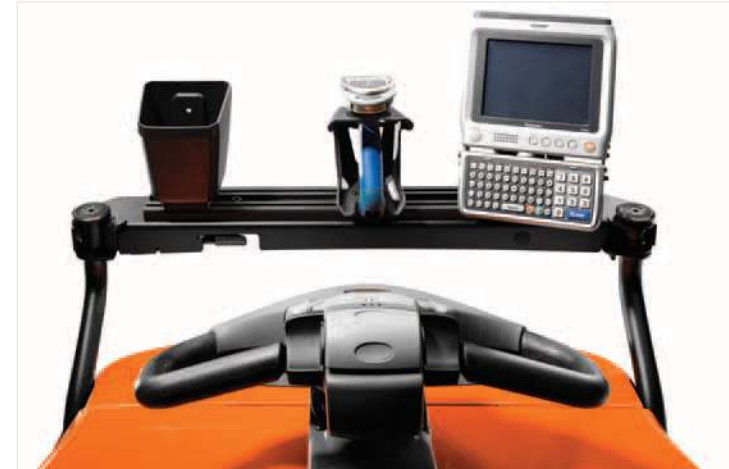
Optional powered E-bar allows easy mounting of ancillary equipment
