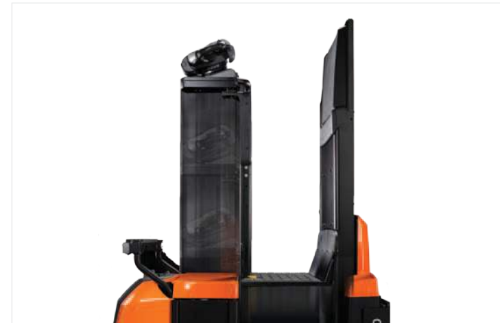
Several models feature platform lift for picking at the second level
