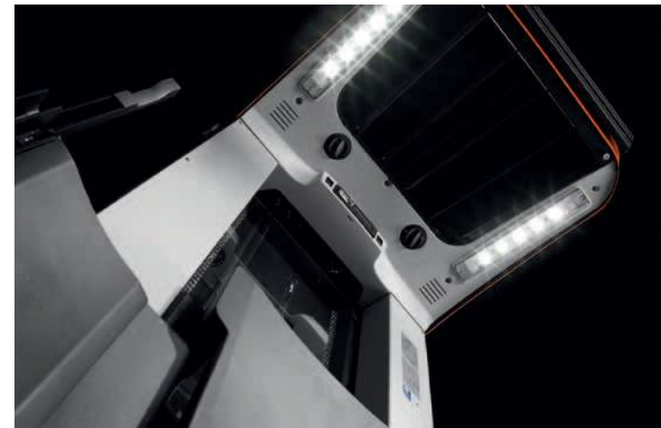
Overhead guard with integral LED working lights
