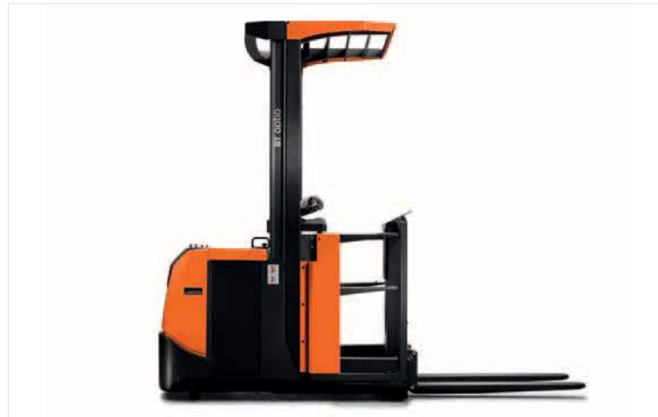
Safety provided by overhead guard
