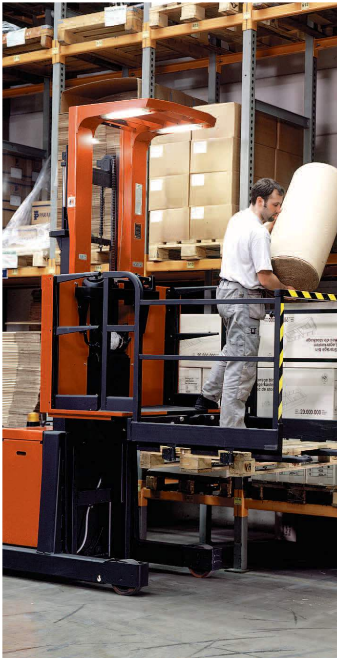
Safety provided by overhead guard
