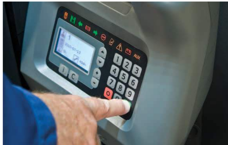
BT Access Control prevents unauthorised use and makes it possible to preset each driver's personal parameters upon start-up
